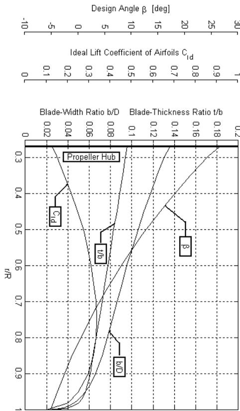
FIGURE 1. Geometry of NACA 4(3)-(08)(03) Blade
