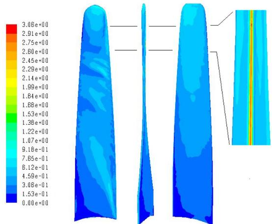
FIGURE 5.  $Y^+$  contours on blade – 2-Blades 4850RPM
