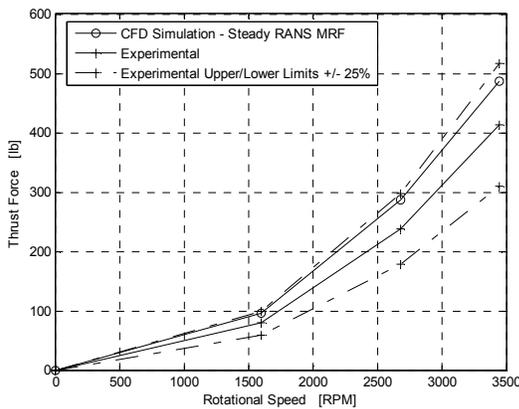
FIGURE 7. Propeller Thrust [lb]
