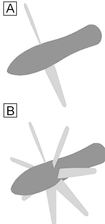
FIGURE 2. NACA 4(3)-(08)(03) Propeller 2-Bladed and 7-Bladed Configurations
