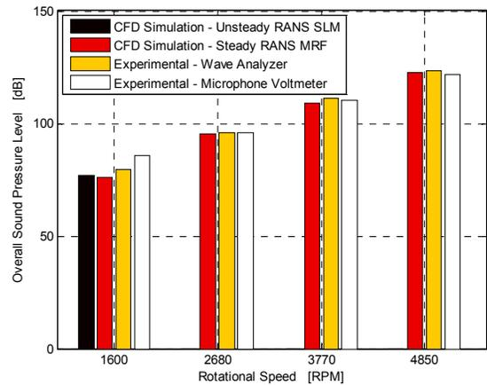
FIGURE 8. Propeller Overall SPL [dB]
