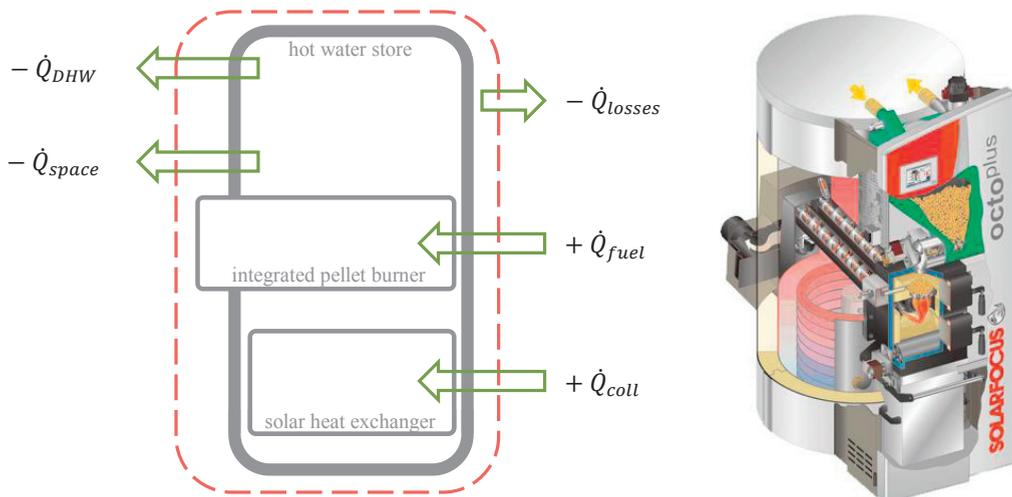
Fig. 1: Investigated system with integrated pellets burner and solar loop heat exchanger (source: SOLARFOCUS GmbH)
