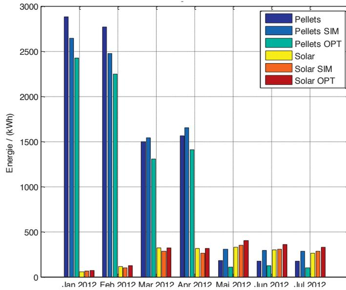
Fig. 2: Monthly biomass energy demand and solar energy supply - Comparison of Monitoring, Simulation and Optimization
