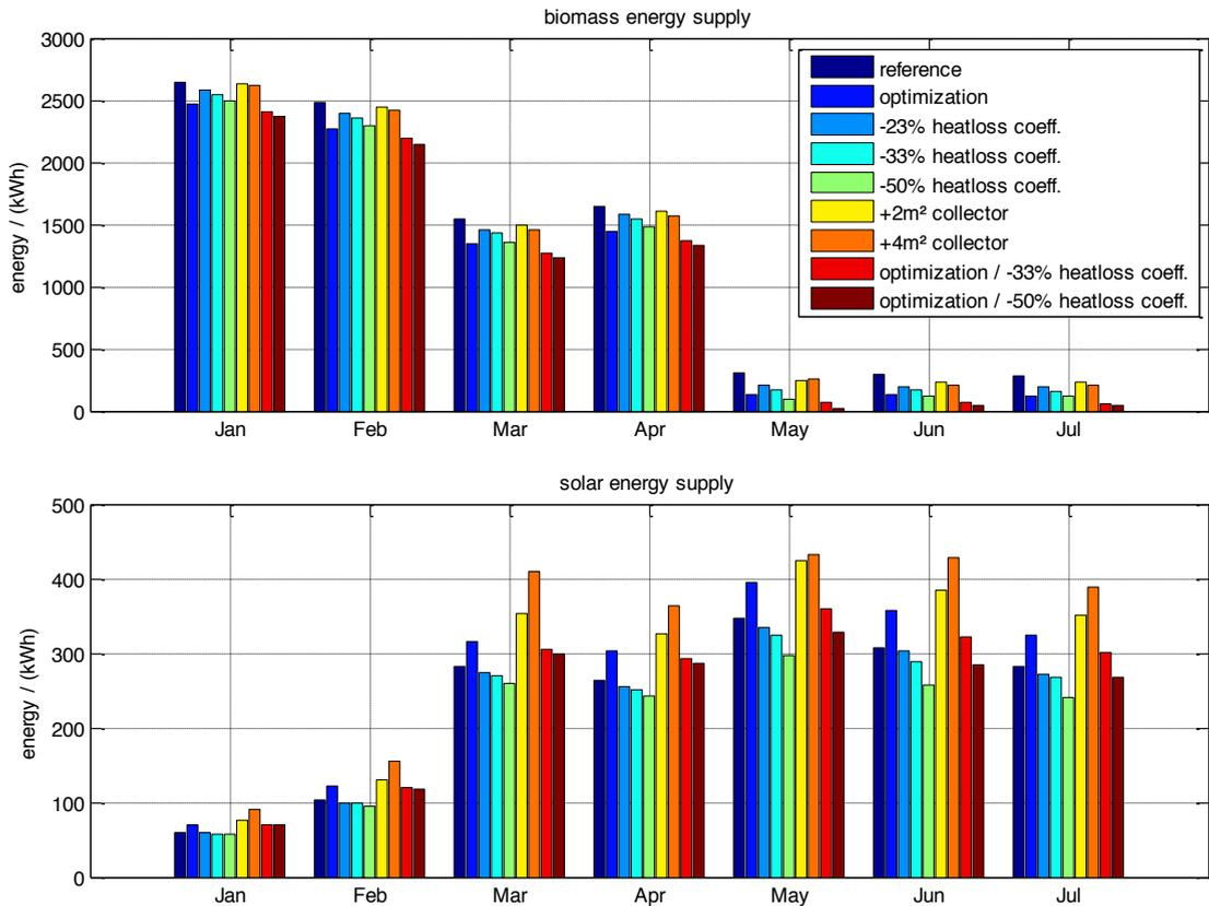
Fig. 3: Simulation Results of the Variation study for both pellet and solar energy supply
