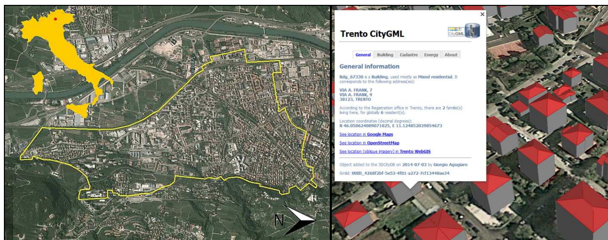
Fig. 2: On the left, the position of Trento in Italy and the extents of the study area. On the right, an excerpt of the 3D city model, visualised in Google Earth. For each building a balloon shows the most relevant data.
