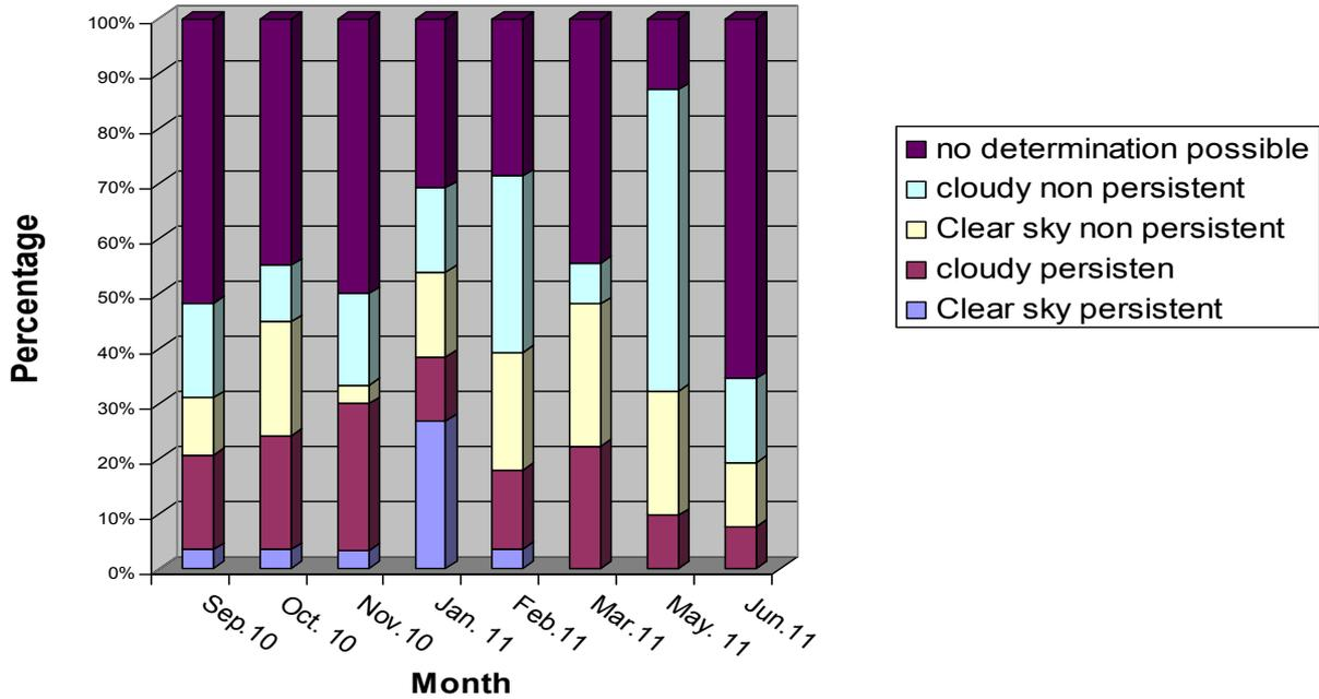
**FIGURE 3.** For each month the percentage of days with and without contrail persistence are shown. Many days (upper part of the columns) mostly with full cloud cover do not allow a determination as to the persistence of contrails. The green and yellow parts of the columns are clear sky and cloudy days without contrail persistence whereas the two lowest partitions of the columns show contrail persistence under cloudy and clear sky conditions.
