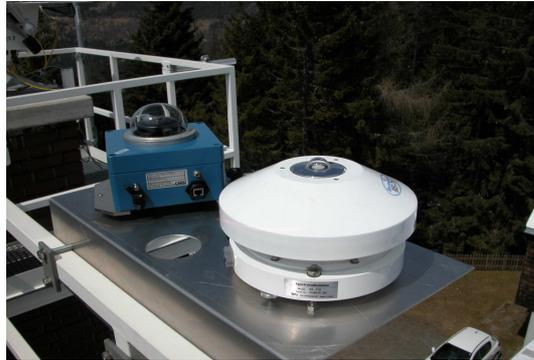
**FIGURE 1.** Fish eye camera (CMS Schreder) (on the left) which performs 1 minute routine photographs of the sky hemisphere with a 180 degree angle of view. On the right hand side an EKO MS 710 Spectrometer may be seen.
