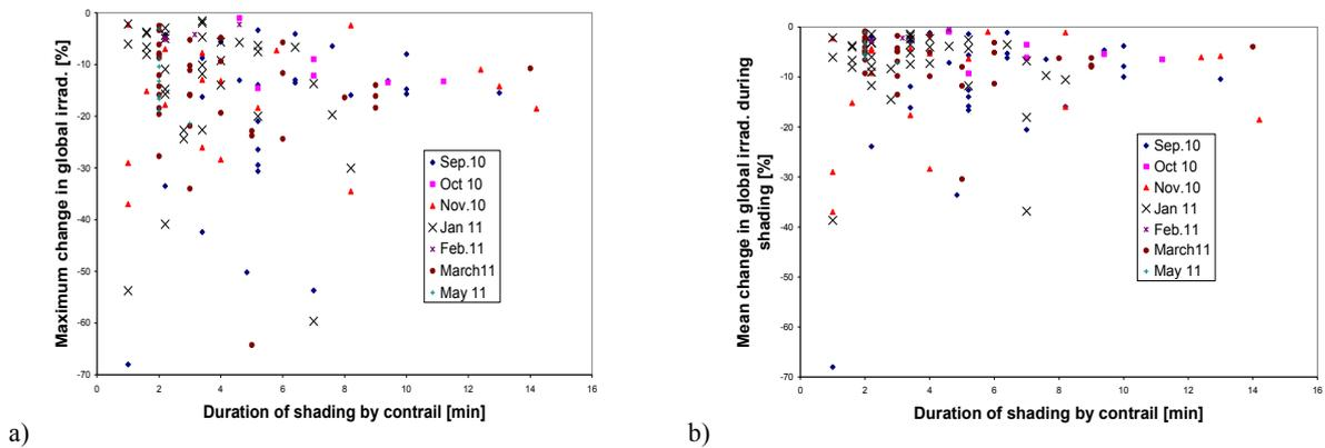
**FIGURE 4.** The maximum **a)** and mean **b)** reduction in global irradiance (during the shading event) as a function of the duration of the shading event by the contrails is shown for the 8 months that were analysed. For June 2011 no shading event was suited for the analysis because of interfering cloudiness which falsified the global irradiance decrease.
