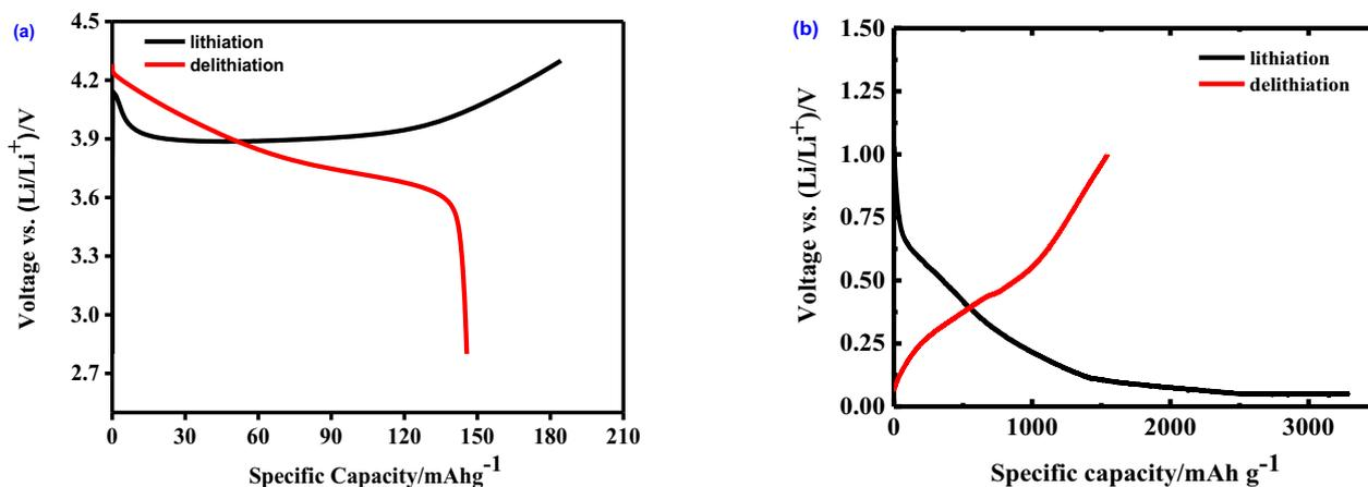
**Figure 1.** (a) 1<sup>st</sup> cycle of voltage vs. specific capacity profiles of NMC532 vs. Li cell cycled in the potential range of 2.8–4.3 V vs. Li/Li<sup>+</sup>; (b) Si/C vs. Li cell cycled in the potential range of 0.05–1 vs. Li/Li<sup>+</sup>.
