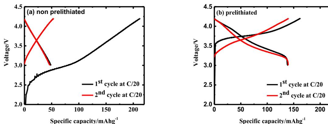
**Figure 2.** Voltage vs. specific capacity profiles of the full cell containing (a) non-prelithiated Si/C and (b) prelithiated Si/C anode at 0.1 V, each coupled with an NMC cathode.
