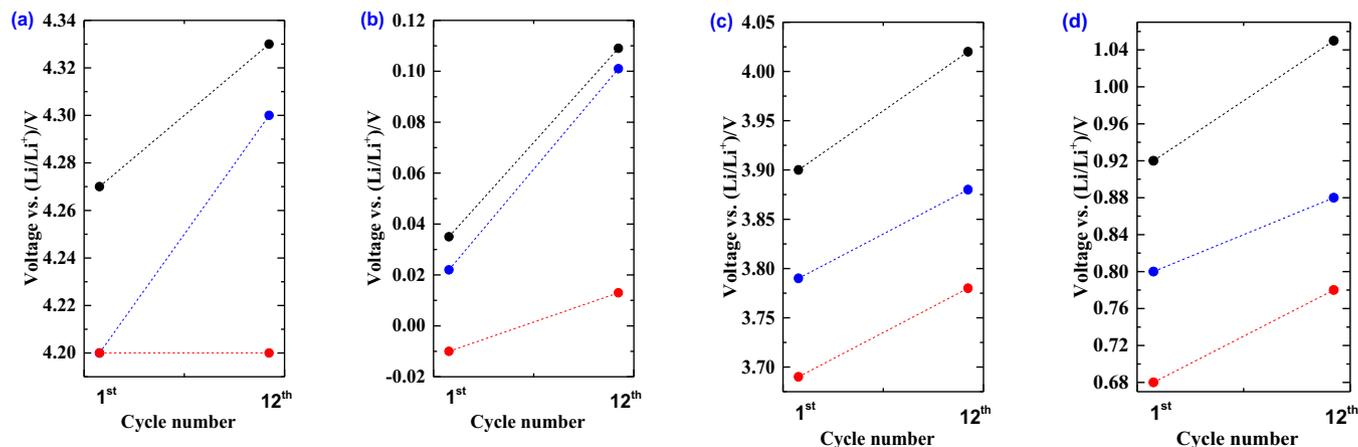
**Figure 5.** (a) Voltage of NCM532 electrodes after cell charge, (b) Si/C electrodes after cell charge, (c) NCM532 electrodes after cell discharge, and (d) Si/C electrodes after cell discharge. The cells containing non-prelithiated Si/C, prelithiated at 0.5 V, and prelithiated at 0.1 V are shown in black, blue and red, respectively.
