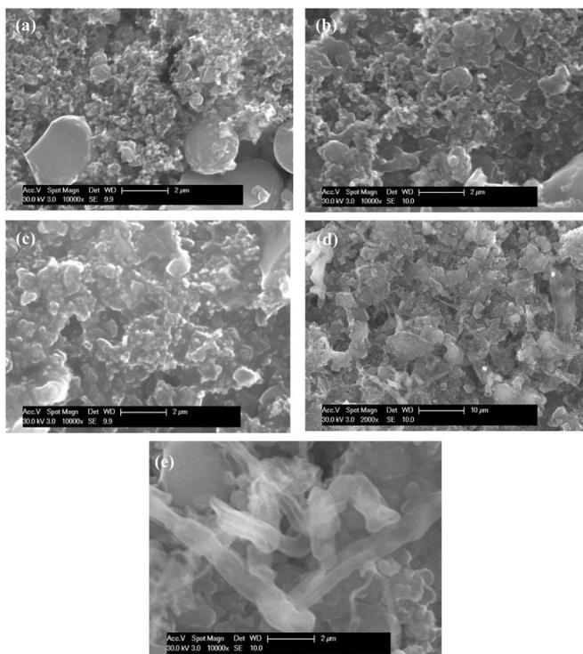
**Figure 7.** SEM images of pristine Si/C electrode (a) before cycling, (b) after cycling and non-prelithiated, (c) prelithiated at 0.5 V, (d) prelithiated at 0.1 V, and (e) appearance of lithium dendrites on the prelithiated at 0.1 V.
