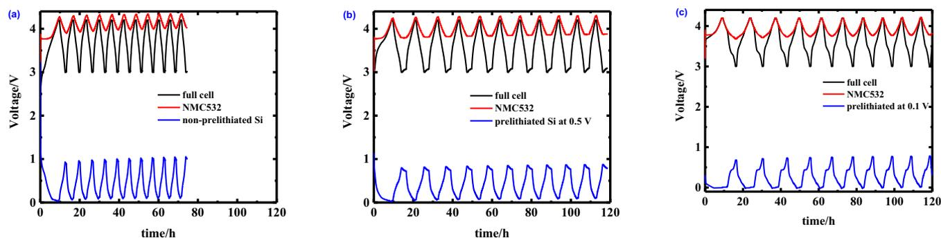
**Figure 4.** Voltage profiles of the overall experiment for the non-prelithiated (a) prelithiated at 0.5 V (b) prelithiated at 0.1 V (c). The red line corresponds to the positive half cell (NMC532), the blue one corresponds to the negative half cell (Si/C), and the black line to the full cell voltages.
