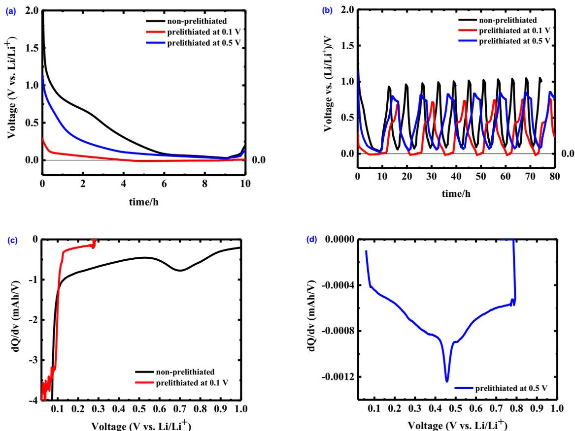
**Figure 6.** Voltage profiles of the Si/C anodes with different degrees of prelithiation for (a) 1<sup>st</sup> cycle, and (b) 10 cycles, dQ/dV vs. voltage profiles of the 1<sup>st</sup> cycle of (c) the non prelithiated and prelithiated at 0.1 V and (d) the prelithiated at 0.5 V.
