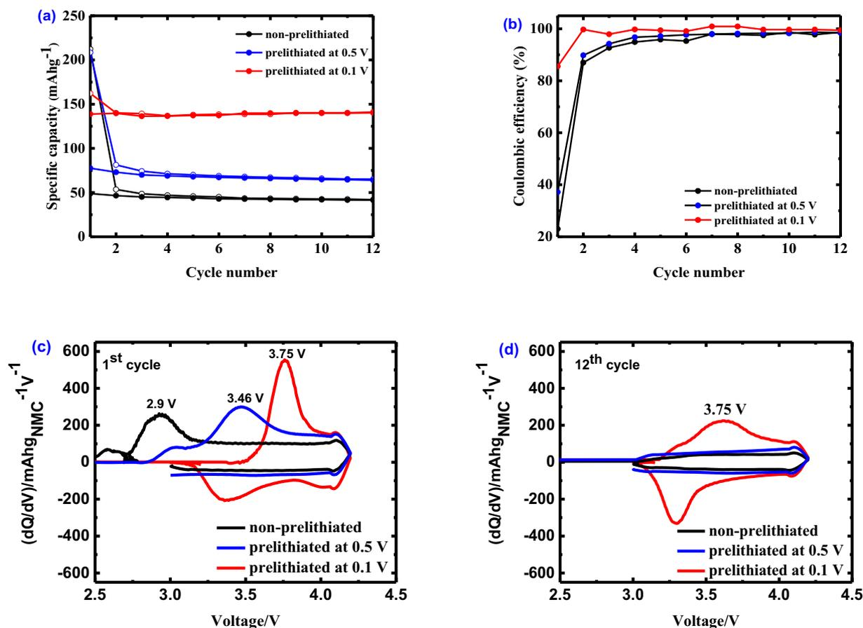
**Figure 3.** (a) Specific capacity and (b) coulombic efficiency vs cycle number profiles,  $dQ/dV$  vs. voltage profiles of (c) the 1<sup>st</sup> cycle and (d) the 12<sup>th</sup> cycle of the full cells containing NMC532 cathodes with Si/C anodes with different degrees of prelithiation in two-electrode set-up.
