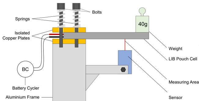
Fig. 1: Functional diagram of the test set-up
