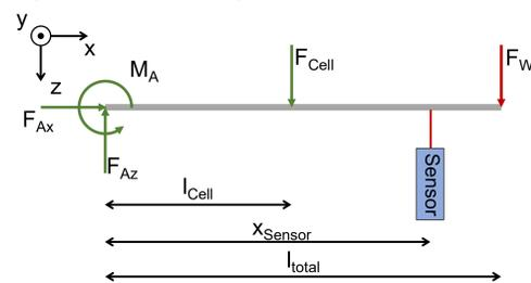
Fig. 2: Diagram of the forces and loads resulting on the LIB
