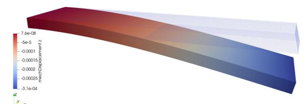
Fig. 5: FEM-Simulation model of the two-point bending test using the software openCFS, visualized in ParaView. (Displacement amplified by the factor 100.)
