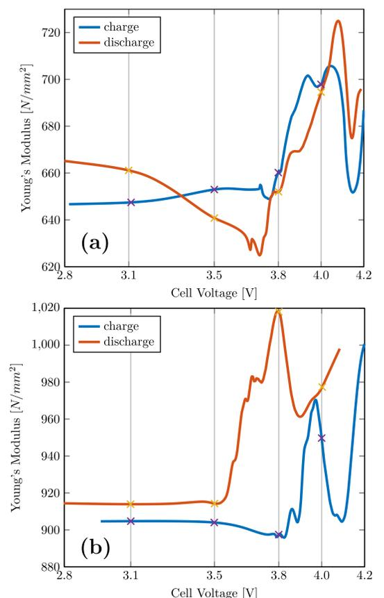
Fig. 4: Mean homogeneous YM for 0.05C (a) and 0.5C (b) with marked YM-values for certain cell voltages which are used for FEM-simulation
