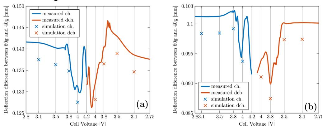
Fig. 6: Measured and simulated deflection for two different weights and two different C-rates, 0.05C (a), 0.5C (b). Using the obtained values for the homogeneous YM from Fig. 4 and a Poisson's ratio of 0.30 for the simulation.
