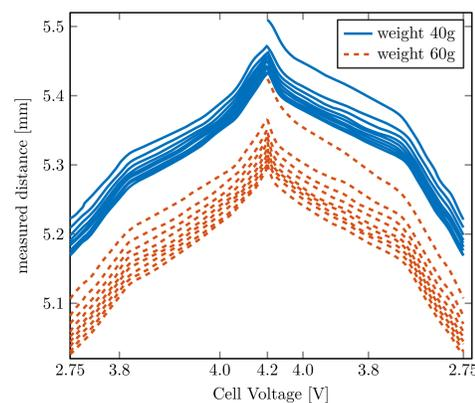
Fig. 3: Measured distance using two different weights over multiple cycles at 0.05C.
